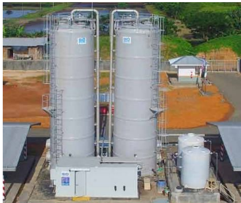
Gambar: Kolom scrubber biogas (Sumber—biogasclean.com).
